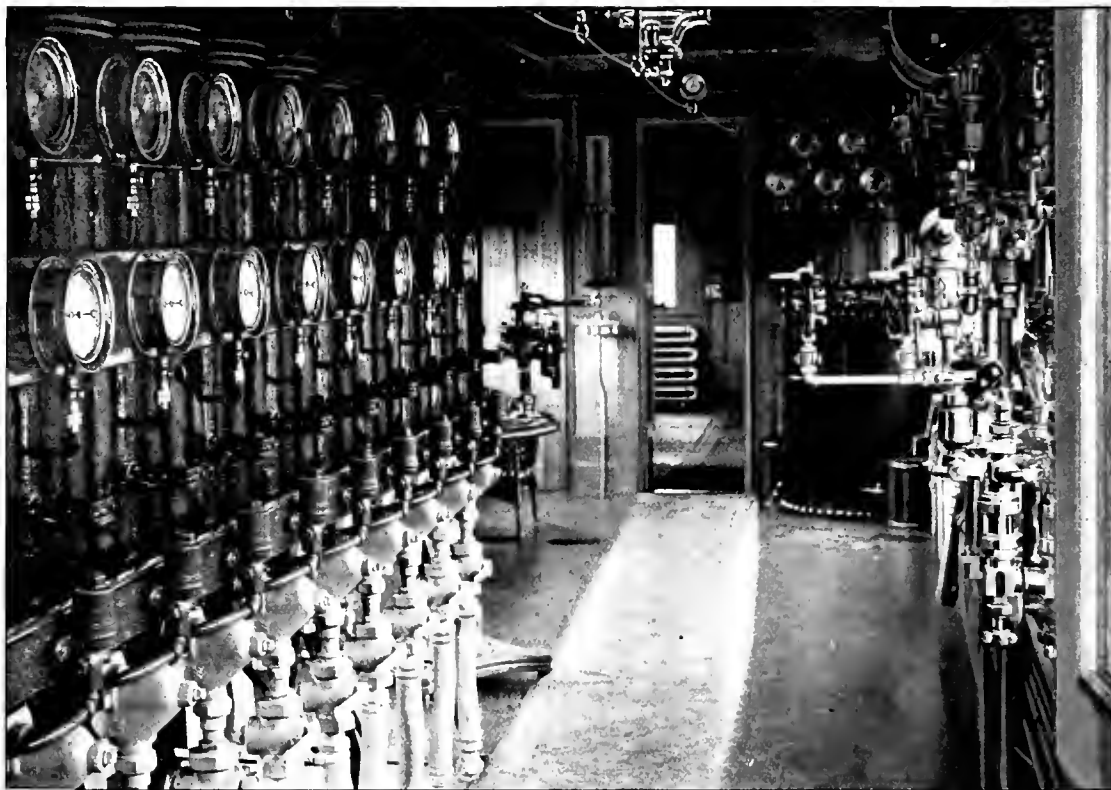
INTERIOR VIEW OF THE N. Y., N. H. & H. AIR BRAKE INSTRUCTION CAR LOOKING TOWARD OFFICE AND SHOWING LIBERAL USE OF GAGES ON CYLINDERS AND AUXILIARIES
